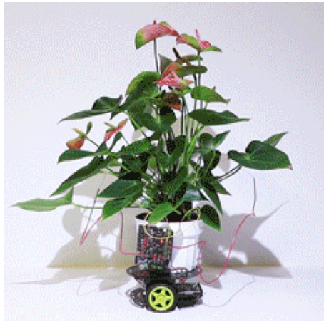
FIGURE 2 Elowan: a plant-robot hybrid. An example of a plant endowed with a wheeled robotic body that can be used to follow a light (credit: Harpreet Sareen, CC BY 4.0, figure adapted from Sareen & Tiao, 2018).
